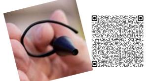
This study seeks to develop a non-invasive communication tool for people with MND and other neuro-disabilities. The EarSwitch sensor is located in the person's ear and is similar to an earbud. An electronic sensor is positioned in either ear canal and monitors for small voluntary movements of the eardrum, sending these signals to software on a computer, phone or compatible assistive device.
